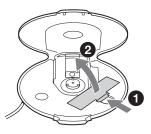
2 Insert the rechargeable battery by matching the ⊕ to the diagram in the battery compartment and close the lid until it clicks into place.
